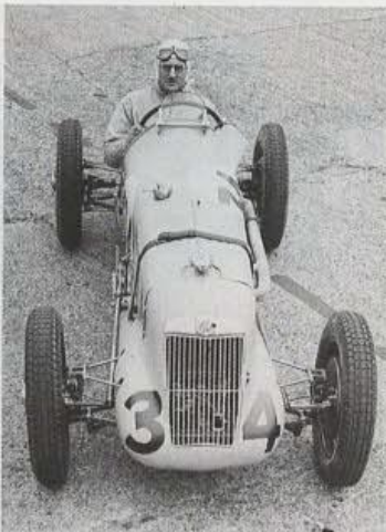
George Eyston in the 1935 International Trophy race car. Note the bulbous front end cowl which MG patented.
