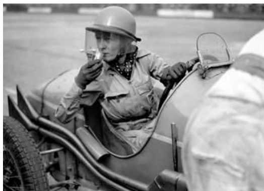
Doreen Evans in R0253 at Brooklands in 1936. At this time RA 0253 was developing 141 bhp at 7,300 rpm with a 25psi boost
